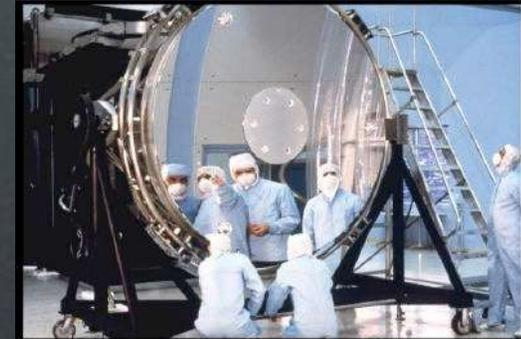
Reflector surface tolerance is dictated by the observing wavelength, and it is usually quoted as a fraction of the observing wavelength.
