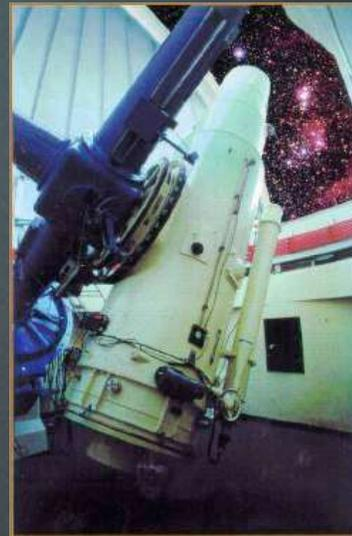
The Schmidt telescope has a spherical primary mirror, and an aspherical correcting lens, known as a corrector plate, located at the radius of curvature of the primary mirror. The detector is placed inside the telescope, at the prime focus.
