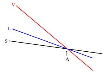
At the *triple point* (A) the molar Gibbs functions of all three phases are equal, and all three phases are in equilibrium. As you increase the temperature from below A to above A, the substance sublimates directly from solid to vapour, as can also be seen from figure VI.5.
