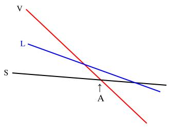
At temperatures below A, the Gibbs function is lowest for the solid, and that is the stable phase. At temperature above A, the Gibbs function is lowest for the vapour, and that is the stable phase. At the pressure represented in the above diagram, the liquid is never the stable phase. The substance sublimates from solid to vapour as the temperature is raised.
