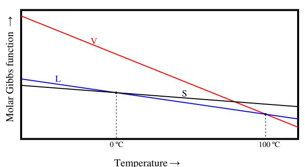
Below 0 °C, the Gibbs function is lowest for the solid, and that is the stable phase. Between 0 °C and 100 °C, the Gibbs function is lowest for the liquid, and that is the stable phase. Above 100 °C, the Gibbs function is lowest for the vapour, and that is the stable phase. At 0 °C, the molar Gibbs function of solid and liquid are equal; the two phases there are in equilibrium. At 100 °C, the molar Gibbs function of gas and liquid are equal; the two phases there are in equilibrium.
