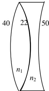
As a result of a manufacturing error, the two types of glass are inadvertently exchanged, and a doublet lens as shown below is made:
