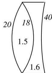
The power, which is the reciprocal of the focal length, is the sum of the powers of the three interfaces:
