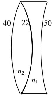
This combination results in an overall *converging* doublet lens of focal length 72 cm.
