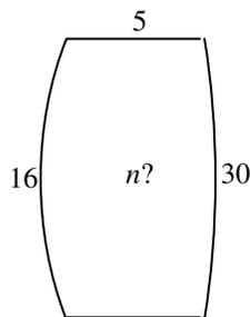
The lens shown has radii of curvature 16 and 30 cm, and is 5 cm thick. An object is 36 cm to the left of the 16 cm face. Its image is 50 cm to the right of the 30 cm surface. Show that the refractive index is the positive solution of
