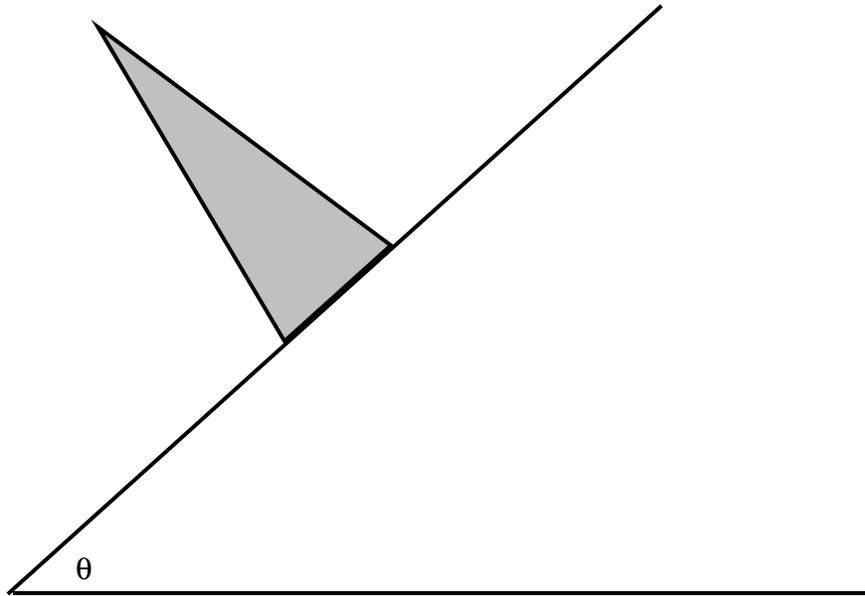
A uniform solid right circular cone of height  $h$  and basal radius  $a$  is placed on an inclined plane whose inclination to the horizontal is gradually increased. The coefficient of limiting static friction is  $\mu$ . Does the cone slip, or does it tip?
