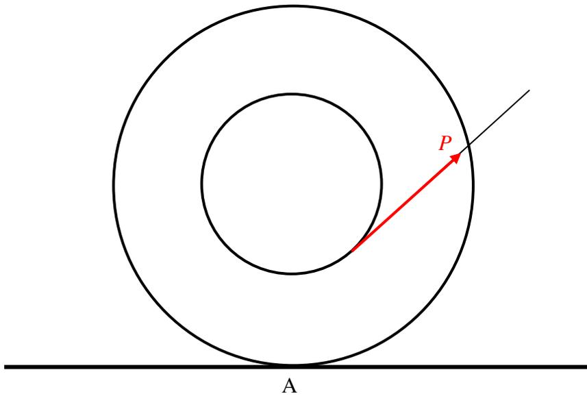
A yo-yo, mass  $M$ , axle radius  $a$ , outer radius  $b$ , rests on a horizontal table as shown. The string, wrapped around the axle, is held at an angle  $\theta$  to the horizontal as shown, and a force  $P$  is applied. The coefficient of friction between yo-yo and table is  $\mu$ .
