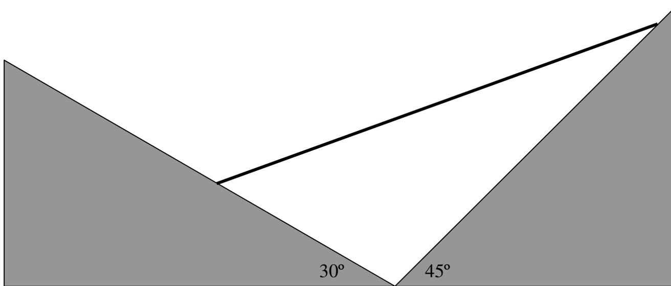
A uniform rod rests on two smooth (frictionless) planes inclined at  $30^\circ$  and  $45^\circ$  to the horizontal. What angle does the rod make with the horizontal?
