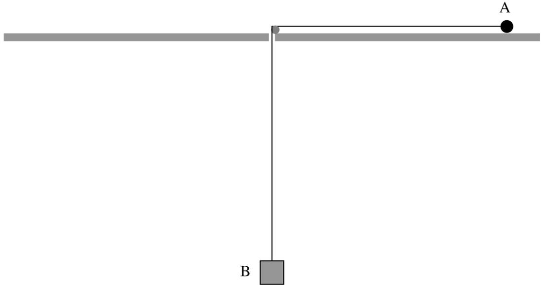
A particle A of mass  $m$  is attached by a light string to a second particle, B, also of mass  $m$ . A rests on a smooth horizontal table, while B hangs vertically through a hole in the table. At time zero, the length of the horizontal portion of the string (i.e. the distance of A from the hole) is  $a$ , and A is moving on the table in a horizontal circle of radius  $a$  with initial angular speed  $\omega_0$ .
