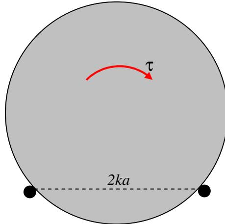
A cylindrical log of diameter  $2a$  and mass  $m$  rests on two rough pegs (coefficient of limiting static friction  $\mu$ ) a distance  $2ka$  apart. A gradually increasing torque  $\tau$  is applied as shown. Does the log slip (i.e. rotate about its axis) or does it tip (about the right hand peg)?
