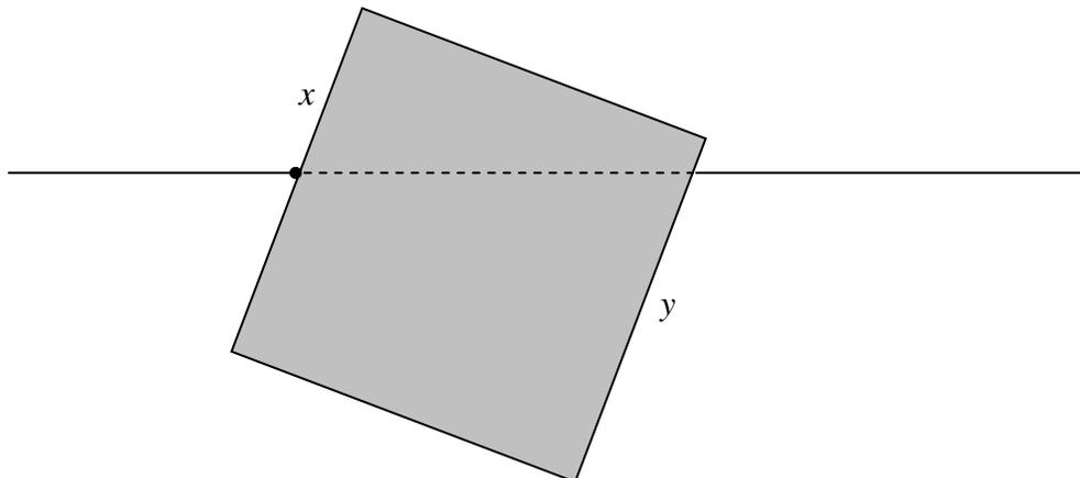
A wooden cube floats on water. One of its faces is freely hinged to an axis fixed in the surface of the water. The hinge is fixed at a distance from the top of the face equal to  $x$  times the length of a side. The opposite face is submerged to a distance  $y$  times the length of a side. Find the relative density  $s$  (that is, relative to the density of the water) of the wood in terms of  $x$  and  $y$ .
