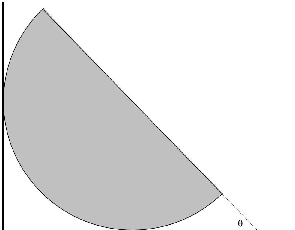
A uniform solid hemisphere of radius  $a$  rests in limiting static equilibrium with its curved surface in contact with a smooth vertical wall and a rough horizontal floor (coefficient of limiting static friction  $\mu$ ). Show that the base of the hemisphere makes an angle  $\theta$  with the floor, where
