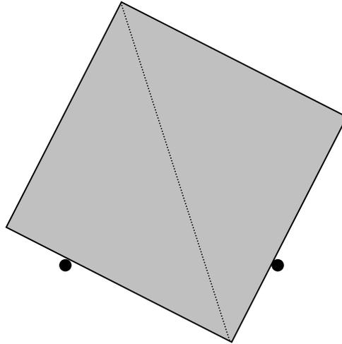
A log of square cross-section, sides  $2a$ , rests on two smooth pegs a distance  $2ka$  apart, one of the diagonals making an angle  $\theta$  with the vertical.
