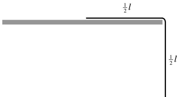
It is released, so that it starts to slide off the table. At a subsequent time  $t$ , a length  $\frac{1}{2}l - x$  remains in contact with the table, the remaining length  $\frac{1}{2}l + x$  hanging vertically, and the speed of the chain is  $v$ :
