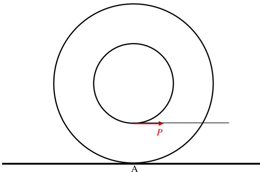
A yo-yo, mass  $M$ , axle radius  $a$ , outer radius  $b$ , rests on a horizontal table as shown. The string, wrapped around the axle, is held horizontally as shown, and a force  $P$  is applied. The coefficient of friction between yo-yo and table is  $\mu$ .
