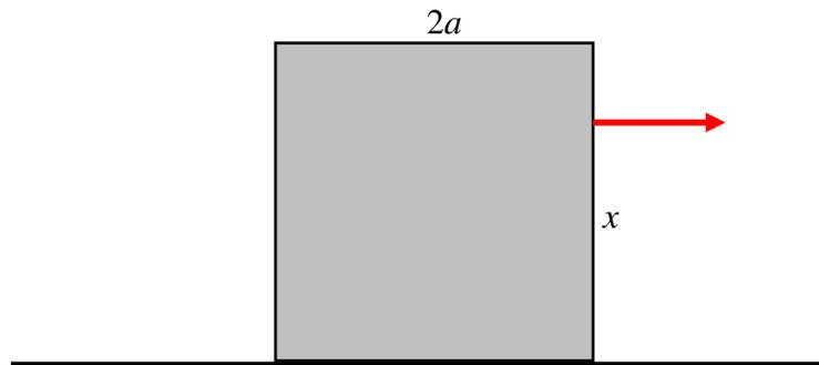
A cubical block of side  $2a$  rests on a rough horizontal table, the coefficient of limiting static friction being  $\mu$ . A gradually increasing horizontal force is applied as shown at a distance  $x$  above the table. Will the block slip or will it tip? Show that, if  $\mu < \frac{1}{2}$ , the block will slip whatever the value of  $x$ .
