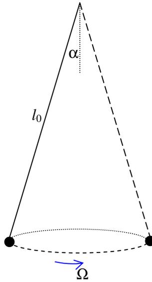
A pendulum of length  $l_0$ , is set into motion so that it describes a cone as shown of semi-vertical angle  $\alpha$ , the bob describing a horizontal circle at angular speed  $\Omega$
