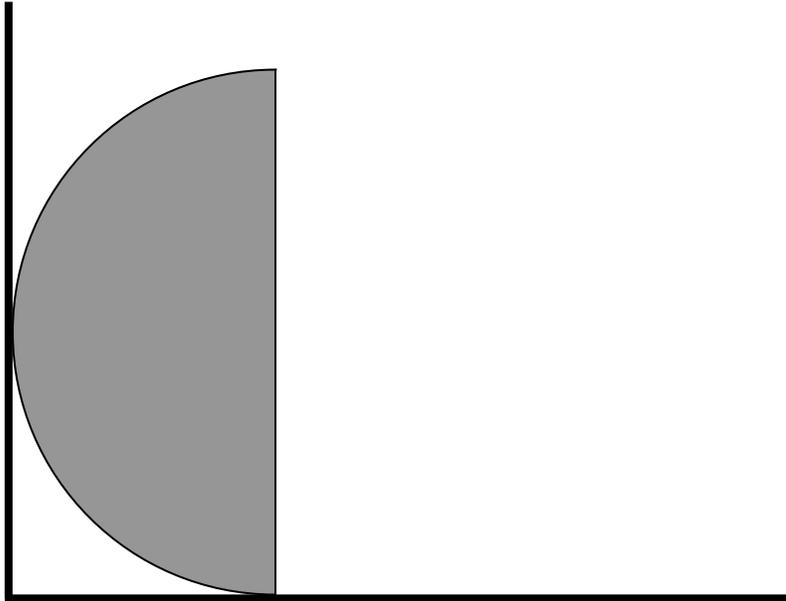
It is then released. Find the reaction  $N_1$  of the floor on the semicylinder and the reaction  $N_2$  of the wall on the semicylinder when its base makes an angle  $\theta$  with the vertical.
