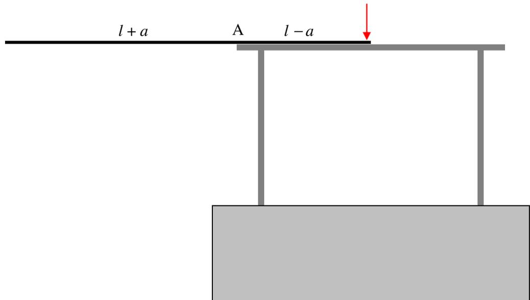
A uniform rod of length  $2l$  rests on a table, with a length  $l - a$  in contact with the table, and the remainder,  $l + a$  sticking over the edge – that is,  $a$  is the distance from the edge of the table to the middle of the rod. It is initially prevented from falling by a force as shown. When the force is removed, the rod turns about A. Show that the rod slips when it makes an angle  $\theta$  with the horizontal, where
