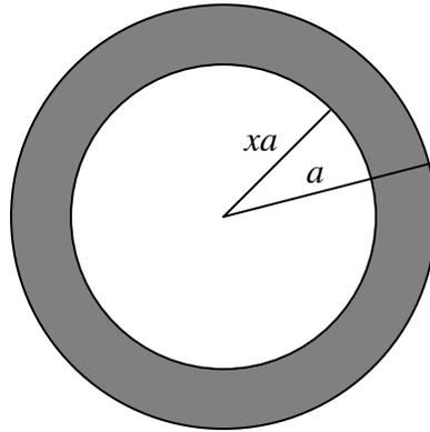
Calculate the moment of inertia of a hollow sphere, mass  $M$ , outer radius  $a$ , inner radius  $xa$ . Express your answer in the form
