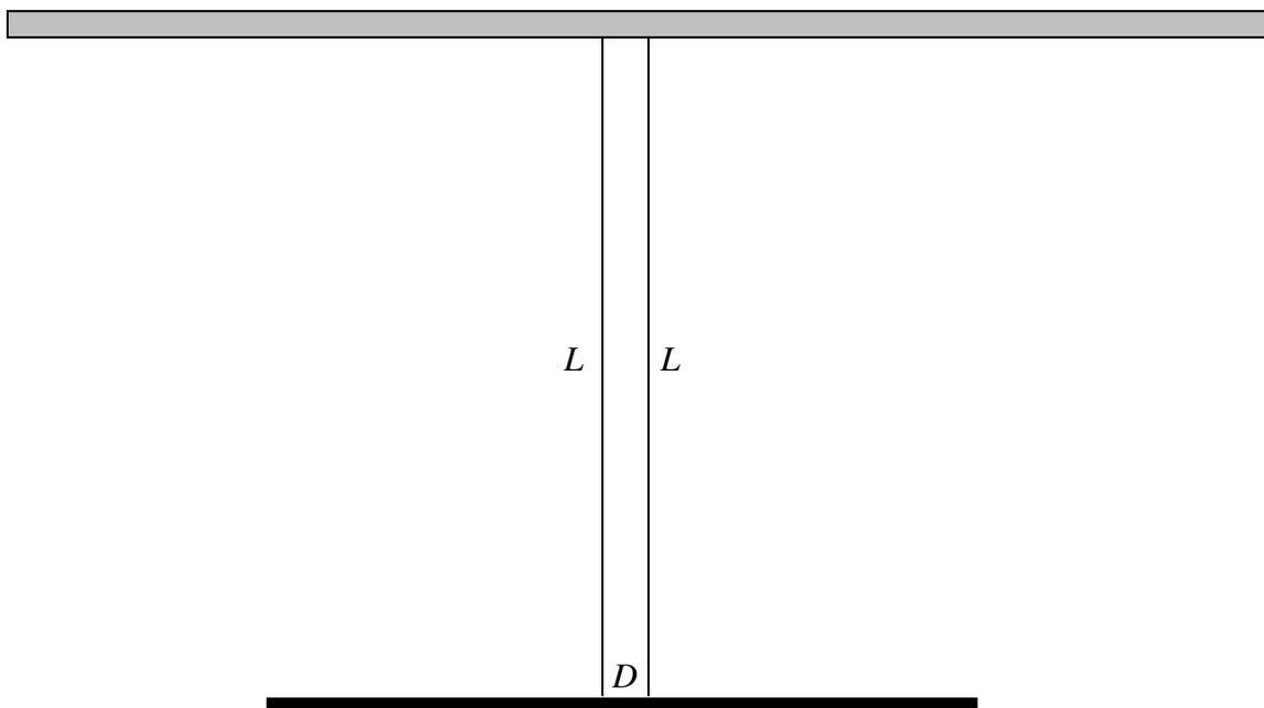
A symmetric but not necessarily uniform rod of mass  $m$  and moment of inertia  $I$  is suspended from the ceiling by two light threads each of length  $L$  a distance  $D$  apart ( $D \ll L$ ). The rod is twisted about a vertical axis through its midpoint through a small angle and then released. Find the period of small oscillations in the horizontal plane.
