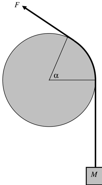
A mass  $M$  hangs from a light rope which passes over a rough cylinder, the coefficient of friction being  $\mu$  and the angle of lap being  $\alpha$ . What is the least value of  $F$ , the tension in the upper part of the rope, required to prevent the mass from falling?
