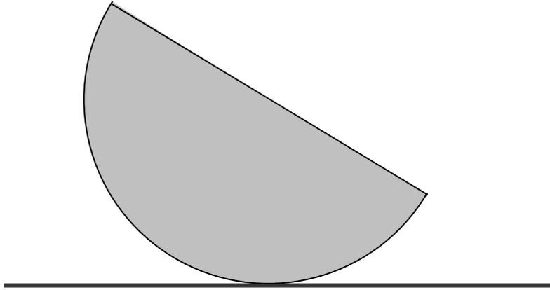
A uniform solid hemisphere of radius  $a$  with its curved surface in contact with a rough horizontal table rocks through a small angle. Show that the period of small oscillations is
