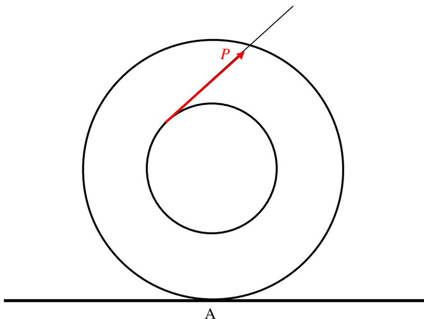
A yo-yo, mass  $M$ , axle radius  $a$ , outer radius  $b$ , rests on a horizontal table as shown. The string, wrapped around the axle, is held at an angle  $\theta$  to the horizontal as shown, and a force  $P$  is applied. The coefficient of friction between yo-yo and table is  $\mu$ .
