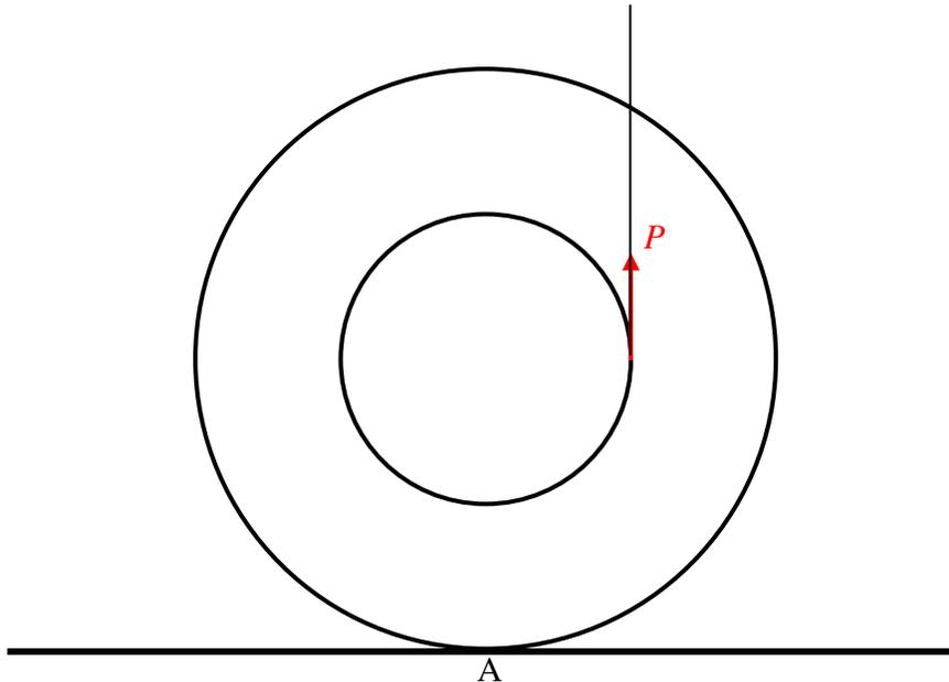
A yo-yo, mass  $M$ , axle radius  $a$ , outer radius  $b$ , rests on a horizontal table as shown. The string, wrapped around the axle, is held vertically as shown, and a force  $P$  is applied. The coefficient of friction between yo-yo and table is  $\mu$ .
