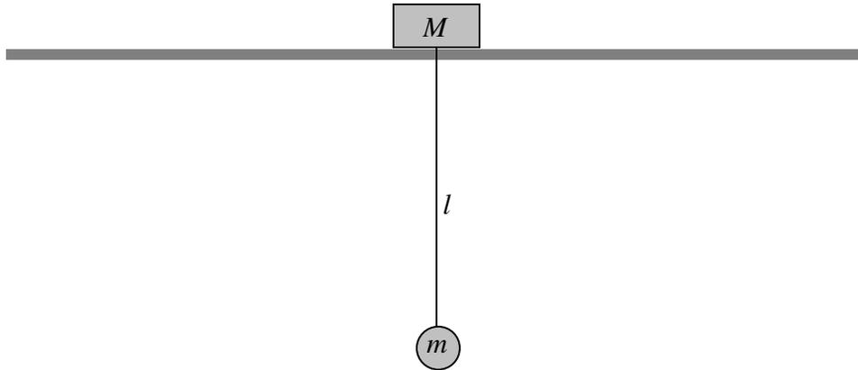
The system is then set in motion with the pendulum swinging, and the mass  $M$  sliding back and forth on the table. At some instant when the horizontal displacement of  $M$  from its equilibrium position is  $x$  the string makes an angle  $\theta$  with the vertical.
