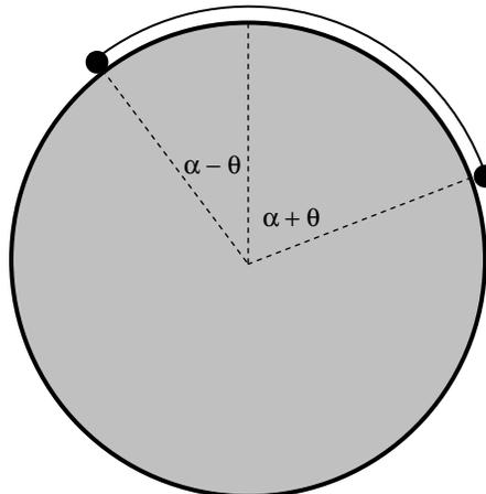
Two identical particles are connected by a light string of length  $2a\alpha$ . The system is draped over a cylinder of radius  $a$  as shown, the coefficient of limiting static friction being  $\mu$ . Determine the angle  $\theta$  when the system is in limiting equilibrium and just about to slide.
