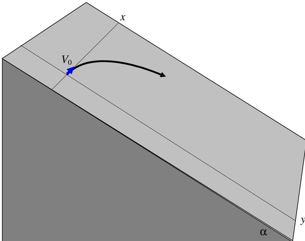
A particle is placed on a rough plane inclined at an angle  $\alpha$  to the horizontal. It is initially in limiting static equilibrium. It is given an initial velocity  $V_0$  along the  $x$ -axis. Ignoring the small difference between the coefficients of moving and limiting static friction, show that at a point on the subsequent trajectory where the tangent to the trajectory makes an angle  $\psi$  with the  $x$ -axis, the speed  $V$  is given by
