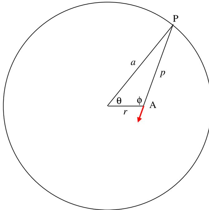
Consider an element  $\delta\theta$  of the ring at  $P$ . The charge on it is  $\frac{Q\delta\theta}{2\pi}$ . The field at  $A$  due this element of charge is
