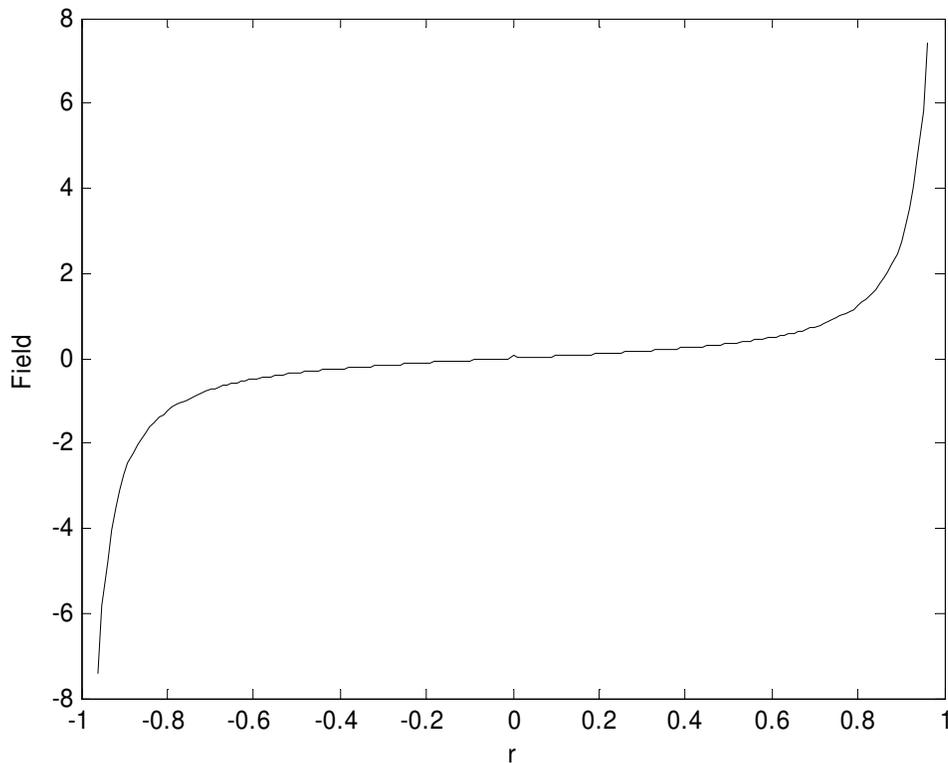
1.6.5 *Field on the Axis of a Uniformly Charged Disc*
