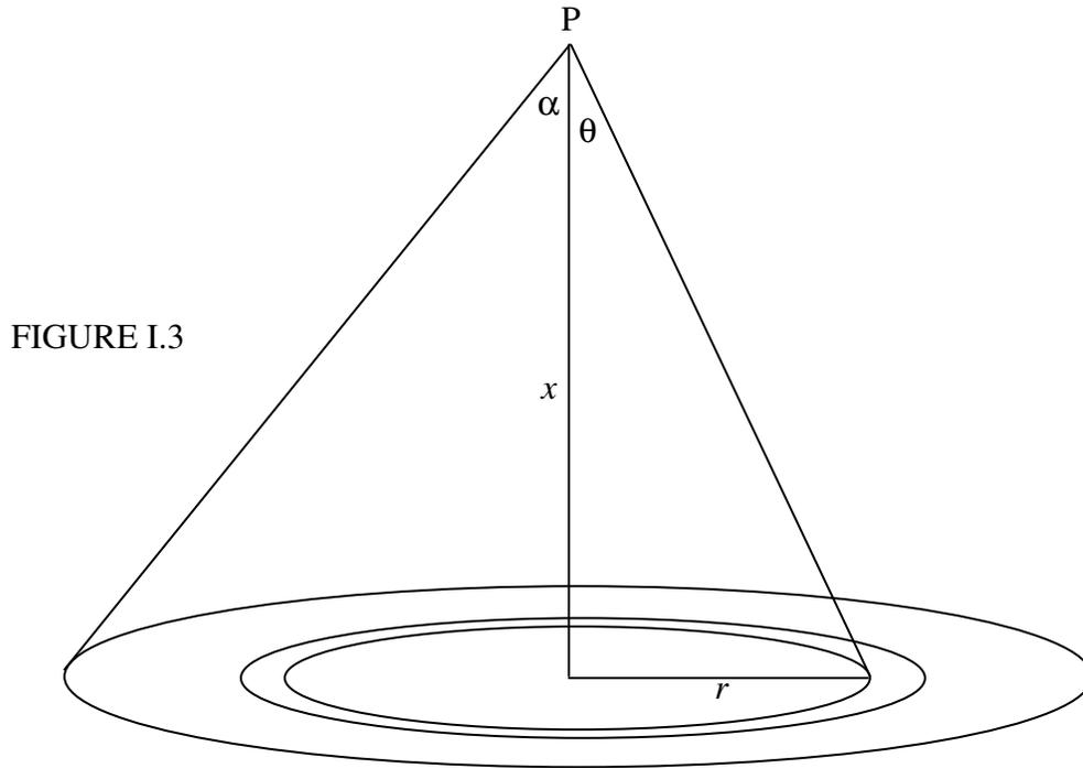
We suppose that we have a circular disc of radius  $a$  bearing a surface charge density of  $\sigma$  coulombs per square metre, so that the total charge is  $Q = \pi a^2 \sigma$ . We wish to calculate the field strength at a point  $P$  on the axis of the disc, at a distance  $x$  from the centre of the disc.
