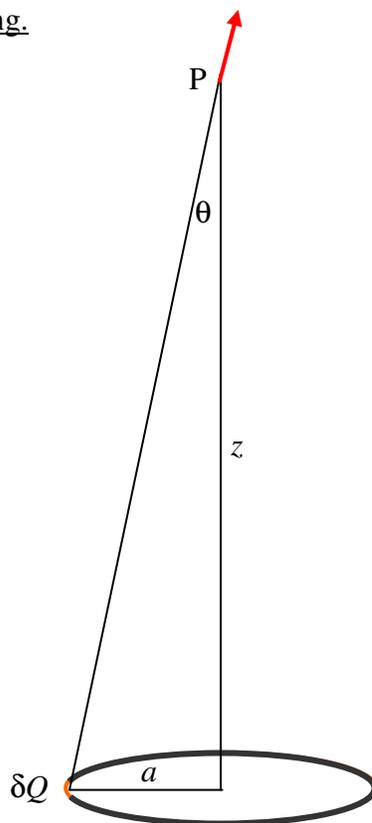
Ring, radius  $a$ , charge  $Q$ . Field at  $P$  from element of charge  $\delta Q = \frac{\delta Q}{4\pi\epsilon_0(a^2 + z^2)}$ .
