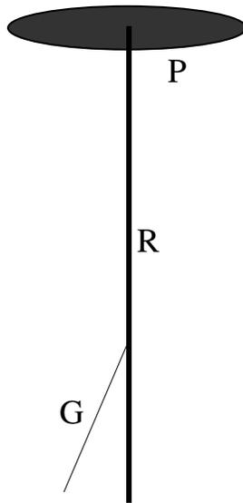
A gold-leaf electroscope has a vertical rod R attached to a flat metal plate P. Gold is a malleable metal which can be hammered into extremely thin and light sheets. A light gold leaf G is attached to the lower end of the rod.
