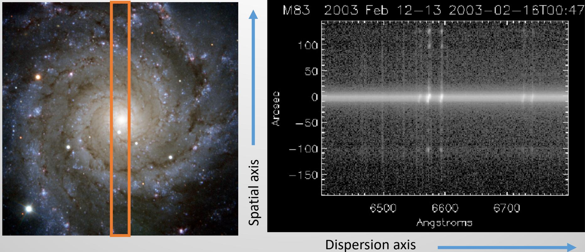
**Long slit spectroscopy (LSS).** A single slit is placed on an extended object and the spectrum is ‘sliced’ in post processing. Quick and cheap, but doesn’t cover whole galaxy. Often used just for rotation curves (edge on galaxies).
