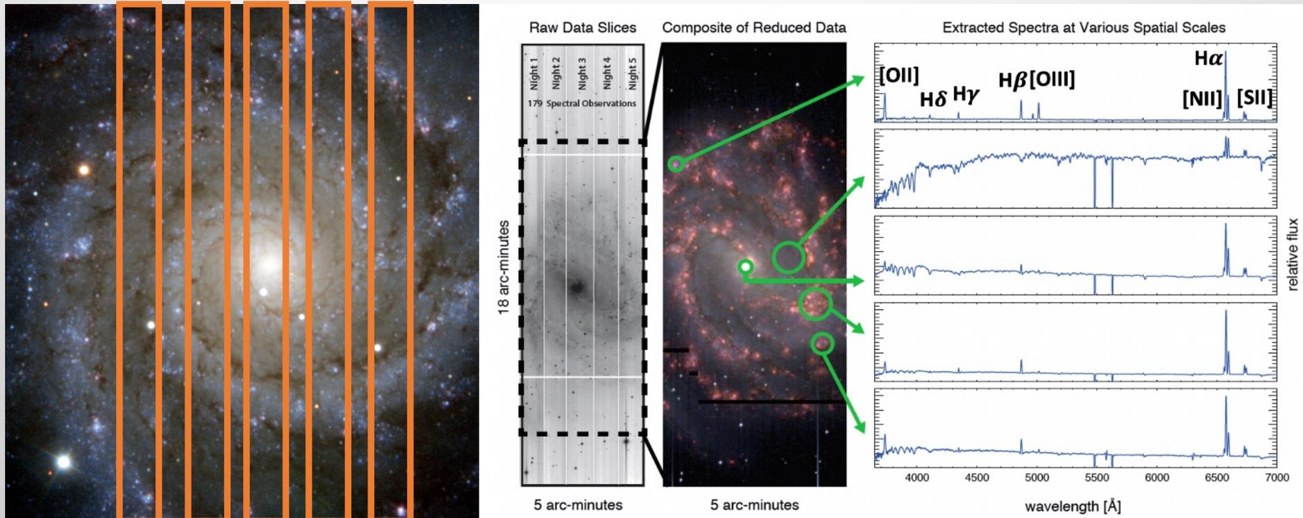
**Multiple LSS** placements (or drift scan). Overlap on CCD means you can only do one LSS at a time. E.g. TYPHOON survey.
