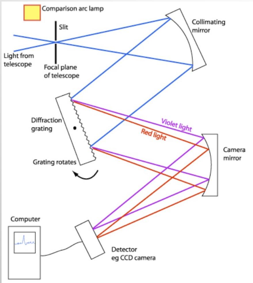
Basic components of a spectrograph:
