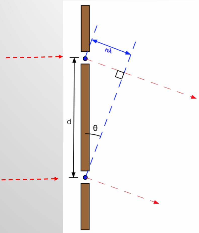
For 2 light rays normally incident on a grating with ruling separation  $d$  the path length is  $d \sin \theta$ .
