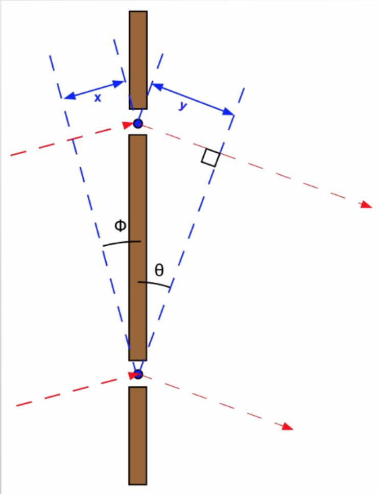
In practice, light rays usually arrive at an angle (not perpendicular) so now the path difference is composed of  $x+y$ :
