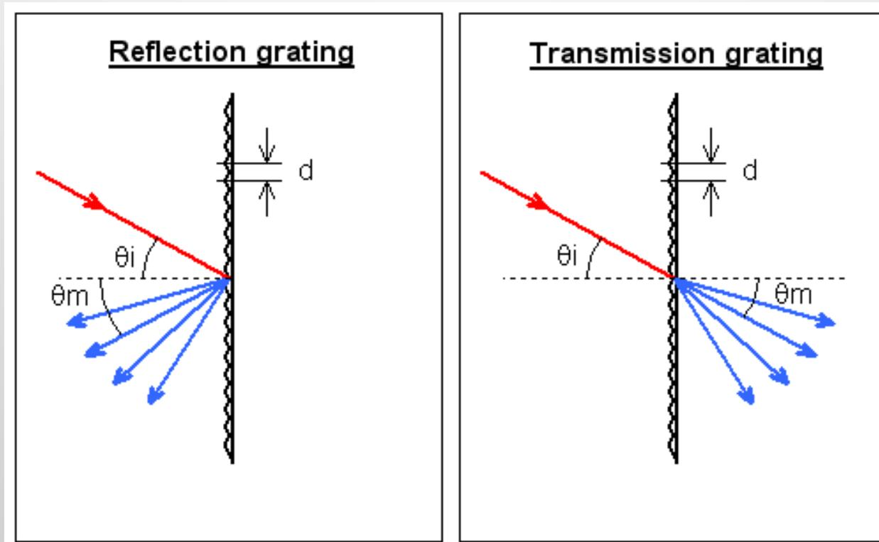
Gratings can be either reflection (reflective surface with grooves) or transmission (transparent surface interrupted by opaque lines).
