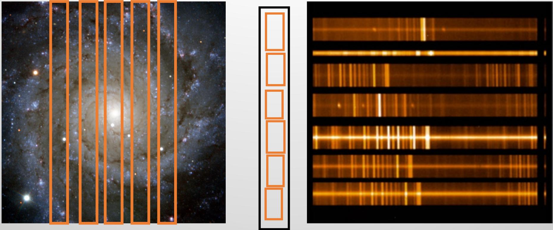
Image is sliced into sections using a segmented mirror. The mirror imaged slices are repositioned on the slit for dispersal.
